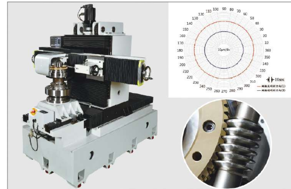
Surface Contact and Pitch Error Testing for Worm Gear System.
